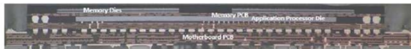
Example of Flip-chip package for APE-Exynos 8 APE in Samsung Galaxy S7 Source: System Plus Consulting APE comparison report
