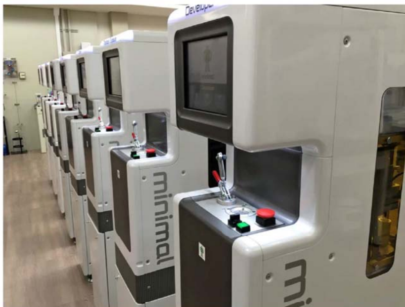
Figure 9-3. Minimal modular wafer fabrication technology
