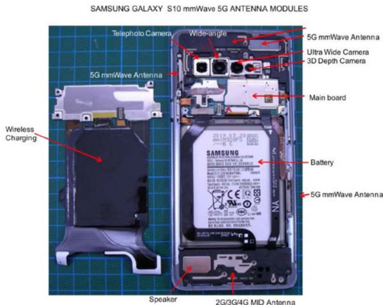
Figure 15. Samsung Galaxy 10 teardown showing 5G antennas. Source: Prismak Partners & Bingahmton University
